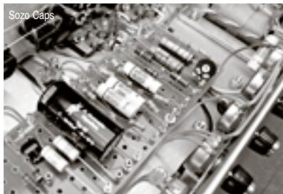
Tone capacitors and coupling capacitors are a huge topic of discussion today. Originally, Marshall used capacitors with film/foil construction. Very early
